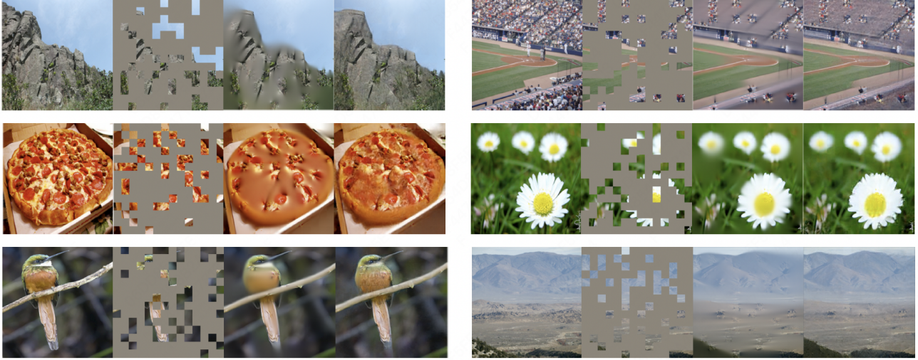
Figure 3. Qualitative analysis for patch reconstruction. Example results are from ImageNet validation set. For each tuple, we show the raw image, masked image, MAE reconstructed image, and our proposed GAN-MAE reconstructed image from left to right. We can see that the reconstructed images from GAN-MAE are significantly clearer than MAE, which we believe benefits the fine-grained visual semantic understanding.
